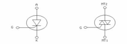
Similar to the SCR, a triac requires a minimum MT2 current to remain in conduction. This minimum current is the holding current.
