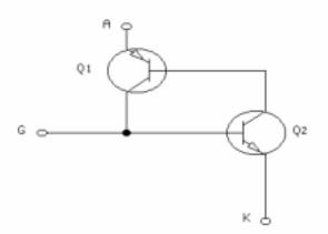
A gate trigger signal turns on transistor Q2. Q2 then forward biases the Q1 base-emitter junction, and both transistors turn on, providing a current path from the anode to the cathode. Both transistors are then latched on until the anode current is removed.
