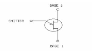
This is the symbol for a **unijunction transistor (UJT)**. The UJT has 1 PN junction and 3 terminals. In this unit, you will use the UJT to control the conduction angle of an SCR.
