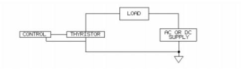
A **thyristor** is a semiconductor device. Electronically controlled switches use thyristors in industrial, military, aerospace, commercial, and consumer applications.
