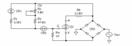
In this circuit, power to the load (R8) can be controlled on both halves of the input cycle. Therefore, the maximum power to the load is twice that of the half-wave circuit.
