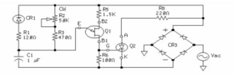
The UJT makes a good trigger device for the SCR because it generates a sharp pulse at the B1 terminal. When the UJT is used with a variable RC phase control circuit, you can easily adjust the phase angle at which the B1 pulse occurs.
