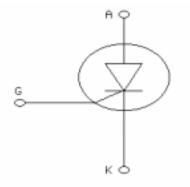
A thyristor is any semiconductor switch. A **silicon controlled rectifier (SCR)** is one type of thyristor. A **silicon controlled rectifier (SCR)** is a 3 terminal, unidirectional thyristor. The 3-terminals are the anode (A), the gate (G), and the cathode (K).
