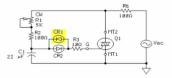
By adding CR1 to the circuit, it becomes a full-wave circuit. Since the triac can conduct on the positive and negative half-cycles, it is bidirectional.
