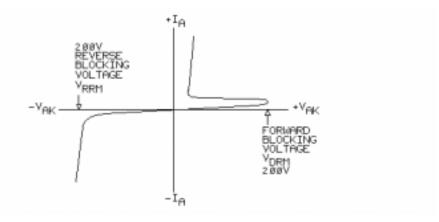
Shown are the voltage/current characteristics of an SCR with no gate current applied and with a forward and **reverse blocking voltage** rating of 200V.
