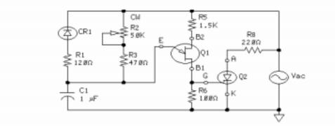
In this circuit, a UJT phase control is used with a half-wave rectifier.
