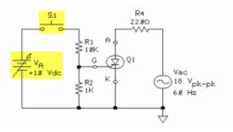
In this circuit, the SCR is a half-wave rectifier that is controlled by S1 and the dc supply  $(V_A)$ . The SCR turns off every negative half-cycle because the SCR becomes reverse biased.
