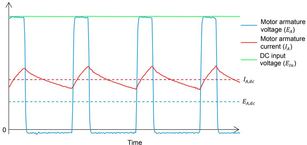
Figure 3. Motor voltage and current waveforms ( $\alpha = 25\%$ ).
