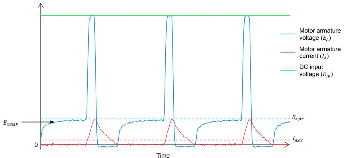
Figure 5. Voltage and current waveforms during deceleration ( $\alpha$  is decreased to 10%).
