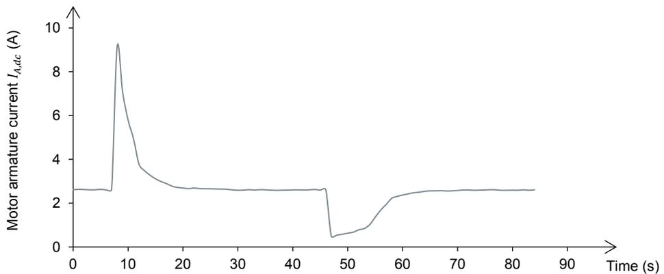
Graphs of the duty cycle, motor speed, and motor armature current as a function of time [Inertia:  $0.100 \text{ kg}\cdot\text{m}^2$  ( $2.373 \text{ lb}\cdot\text{ft}^2$ ), friction torque:  $0.60 \text{ N}\cdot\text{m}$  ( $5.31 \text{ lbf}\cdot\text{in}$ )].
