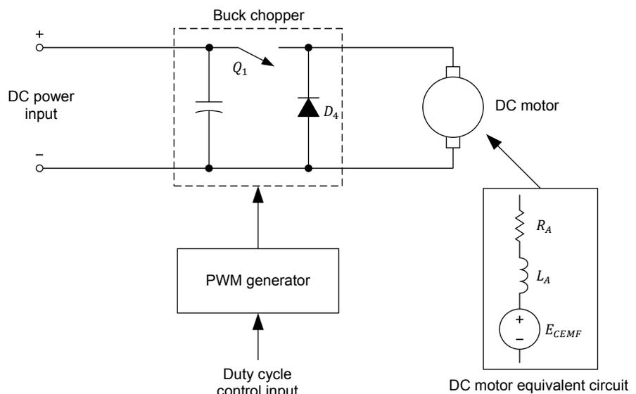
Figure 2. Basic PWM dc motor drive.
