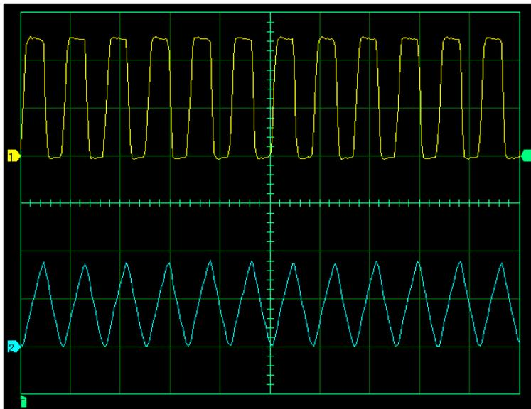
Waveforms of the motor armature voltage and current when operating at  $\alpha = 50\%$ .
