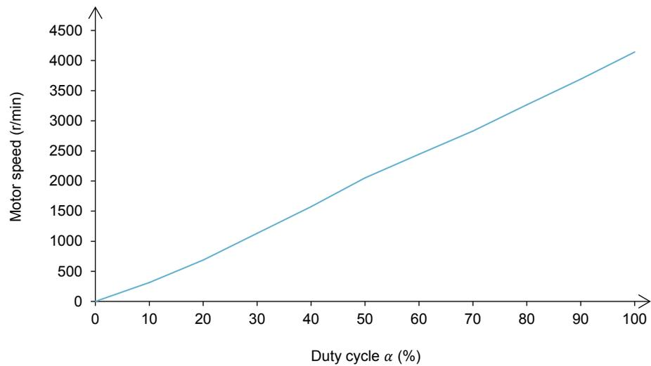
Speed of the dc motor as a function of the duty cycle  $\alpha$  of the buck chopper.
