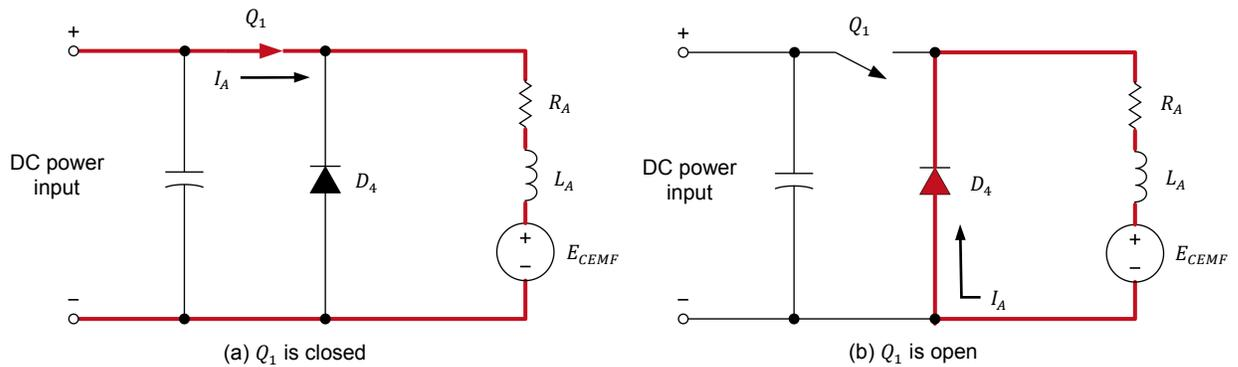
Figure 4. The two paths of the armature current.
