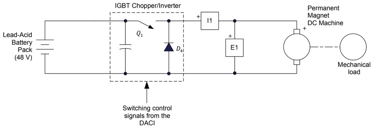
Figure 6. Basic PWM dc motor drive (buck chopper dc motor drive).
