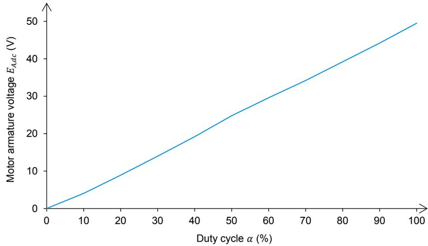
Armature voltage ( $E_{A,dc}$ ) of the dc motor as a function of the duty cycle  $\alpha$  of the buck chopper.
