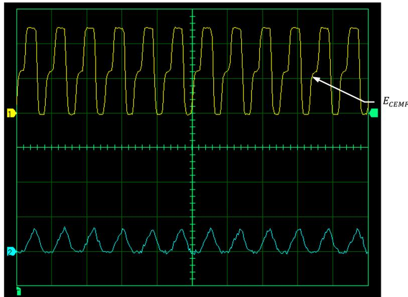
Figure 7. The dc motor counter-electromotive force ( $E_{CEMF}$ ) is visible in the armature voltage waveform during the deceleration.
