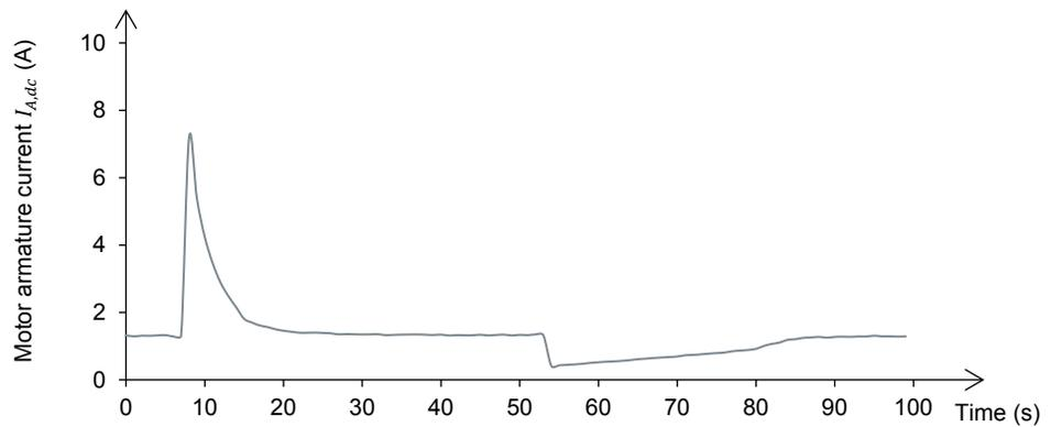
Graphs of the duty cycle, motor speed, and motor armature current as a function of time. [Inertia: 0.100 kg·m<sup>2</sup> (2.373 lb·ft<sup>2</sup>), friction torque: 0.30 N·m (2.66 lbf·in)].
