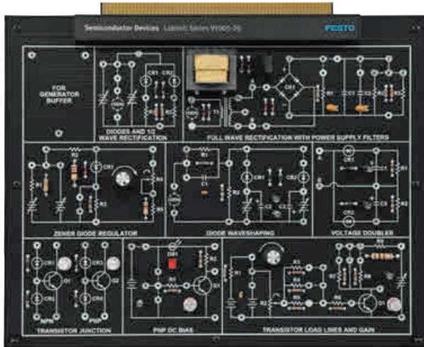
The Semiconductor Devices Circuit Board contains nine circuit blocks pertaining to skills training in semiconductor circuits.
