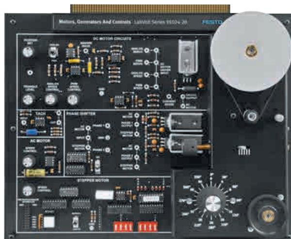
The Motors, Generators, and Controls course provides comprehensive, hands-on instruction in the terminology, principles, and applications of the DC motor, AC synchronous motor, phase shifter, and stepper motor.
