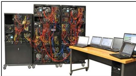
of an actual grid. This setup is also reconfigurable, i.e., all the components can be rearranged for further experiments as the connections are not fixed.
