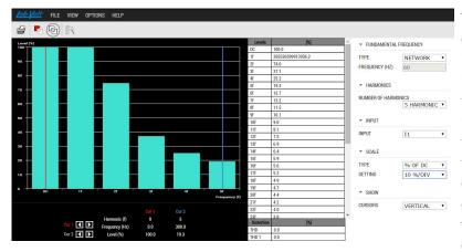
The Harmonic Analyzer allows observation and analysis of the harmonic components in the measured voltages and currents. The fundamental frequency can be manually set to the ac power network frequency or automatically set to the frequency of the fundamental component of the selected voltage or current. The harmonic components of the selected voltage or current can be displayed using a vertical scale
