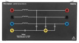
The Three-Phase Filters consists of three inductors and four capacitors enclosed in a half-size EMS module. Eight safety banana jacks on the module front panel provide access to the three-phase filter. The module is used to filter three-phase signals in power electronics applications.
