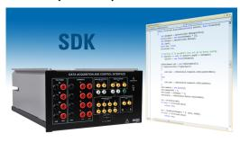
The DACI SDK (Software Development Kit) offers the possibility to control various inputs and outputs of the Data Acquisition and Control Interface using third-party rapid prototyping software like Mathworks® MATLAB, National Instruments® LabVIEW, Microsoft Visual Studio and other programming tools that support Microsoft® .NET Framework 4.0. The SDK gives users the possibility to build their own advanced functions using the Data Acquisition and Control Interface.
