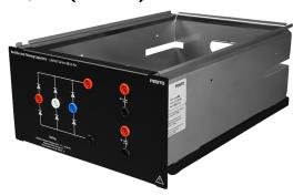
This Rectifier and Filtering Capacitors module consists of a three-phase bridge rectifier and two separate capacitors enclosed in a half-size EMS module. The bridge allows the conversion of a three-phase voltage input into an unfiltered dc voltage. This dc voltage can then be filtered using the polarized capacitors (each one protected by a diode). Internal electrical components are identified on the module front panel by silkscreened symbols and terminated by 4 mm safety banana jacks.
