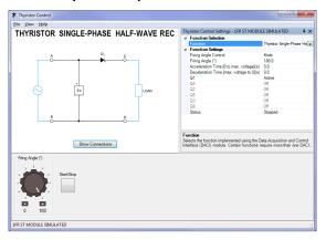
The Thyristor Control Function Set enables the following thyristor-based devices to be implemented using the Data Acquisition and Control Interface, and the Power Thyristors:
