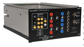
The Power Thyristors module consists of six power thyristors (SCRs) mounted in a half-size EMS enclosure. Each individual thyristor is protected against overcurrents and short-circuits. All the anodes and cathodes of the thyristors are terminated on the front panel by color-coded, 4 mm safety banana jacks. To reduce the number of external connections, the most typical thyristor configurations can be achieved through the use of two toggle switches on the front panel.
