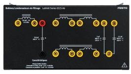
This Filtering Inductors/Capacitors module consists of two separate filters enclosed in a half-size EMS module: a low-frequency filter and a high-frequency filter. The low-frequency filter consists of an inductor and a polarized capacitor, while the high-frequency filter consists of two inductors and a non-polarized capacitor. Internal electrical components are identified on the module front panel. 4 mm banana jacks provide access to the different components in the module.
