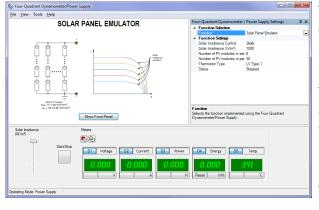
The Solar Panel Emulator Function Set is a function that can be activated in the Four-Quadrant Dynamometer/ Power Supply enabling the module to emulate a solar panel.
