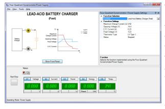
The Lead-Acid Battery Charger Function Set is a package of control functions that can be activated in the Four-Quadrant Dynamometer/Power Supply, enabling the module to implement a lead-acid battery charger, as well as a battery discharger.
