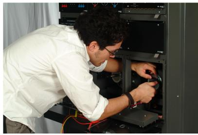
All rotating machines are mounted in standard-size modules. These modules are equipped with a clear plastic faceplate fitted with a chrome-plated piano hinge. The faceplate can be lowered for access to the machine, and when closed, it is secured by two quick-lock fasteners. Each rotating machine is provided with a safety locking device that prevents students from lowering the faceplate during lab exercises.
