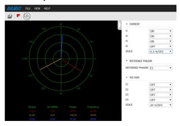
The Phasor Analyzer displays the phasors related to the measured voltages and currents. The amplitude and phase angle of each voltage and current is clearly represented by the orientation and length of their corresponding phasors, allowing easy comparison between the displayed parameters. This produces a unique and dynamic display of the voltages and currents in a circuit (especially in three-phase circuits) that cannot be obtained with conventional
