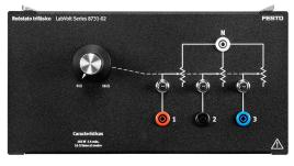
The Three-Phase Rheostat module consists of three rheostats mounted on a common shaft directly controlled by a single knob on the module faceplate. The rheostats are electrically interconnected in a four-wire wye configuration and each leg is protected from over-current conditions by a thermal-magnetic circuit breaker.
