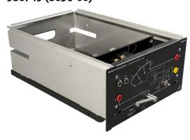
The Manual DC Motor Starter can be wired as either a three or four point dc starter to be used in conjunction with the DC Motor/Generator, Model 8211. The module has a fitted, manually operated handle for variable resistance starting. When it is in the full-run position, the handle is held in place by an electromagnet. In the event of field loss, the holding electromagnet is de-energized and the starting handle is returned to the off position by a stiff spring.
