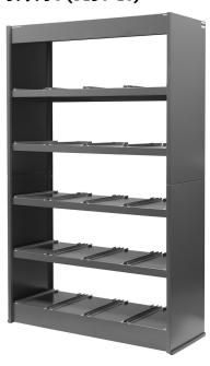
The Storage Shelves module contains five shelves, each of which can accommodate four full-size EMS modules or eight half-size EMS modules. Stainless steel rails guide the modules on the storage shelves and protect them against wear. The Storage Shelves module requires assembly. A diagram is provided to facilitate assembly. Note that this model cannot stand by itself and must be attached to a wall.
