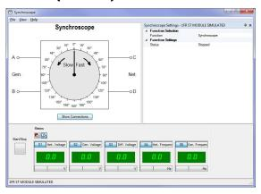
The Synchroscope Function is used for the synchronization of synchronous generators. This function emulates the operation of an actual synchroscope by showing on-screen the dial indicating the phase angle difference between the generator voltage and the network voltage. In addition, the Synchroscope Function includes meters displaying various parameters important to generator synchronization (e.g., network voltage and frequency, generator voltage and frequency, voltage difference).
