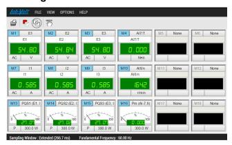
The Metering window displays up to eighteen meters, which can be configured individually for measuring ac/dc voltage and current, electrical power (active, reactive, and apparent), torque, speed, mechanical power, etc. The voltage and current meters have several modes of operation that allow measurement of the mean (dc) value, RMS value, crest factor, RMS value of a particular harmonic (up to the 15th
