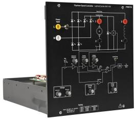
The Thyristor Speed Controller is designed to control the speed of the DC Motor/Generator in both the open-loop and closed-loop modes of control.
