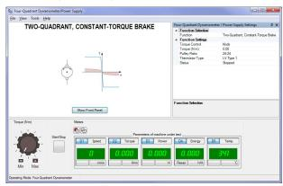
The Standard Functions (computer-based control) Set is a package of control functions that can be activated in the Four-Quadrant Dynamometer/Power Supply, enabling the module to perform a wide variety of functions in each of its two operating modes (Dynamometer and Power Supply).
