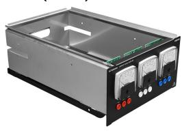
The AC Voltmeter module is fitted with three separate multirange ac voltmeters for simultaneous measurement of threephase voltages. Meter ranges and scalar values of each instrument have been carefully selected for compatibility and are appropriate for the electrical values to be measured. All meter readings are direct indications and do not require the indicated value to be mentally multiplied by a constant.
