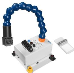
The Polarized Retroreflective Photoelectric Switch consists of a light source and a receiver combined in the same casing. This sensor requires a special retroreflective surface. The sensor is mounted on a flexible support for easy positioning. The model has one normally open and one normally closed contact, and the electrical connections are made using either the banana jacks or the terminal block.
