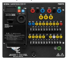
The AC Drive consists of a variable frequency speed drive with V/ Hz control. The AC Drive has programmable inputs and outputs, digital and analog (for PID Control). Some electrical connections can be made using either the banana jacks or the terminal blocks.
