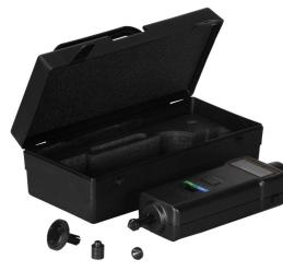
The Digital Tachometer indicates motor rotation speed either in a clockwise or counterclockwise direction. The measured speed is automatically indicated on a five-digit display and is updated every second to enable measurement of acceleration and deceleration.
