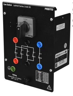
The Cam Switch consists of a manually operated drum switch. The switch control lever has three positions: Off, Forward, and Reverse. The Cam Switch is suitable for both single-phase and three-phase ac motor control. It can also be used to control series and compound dc motors.
