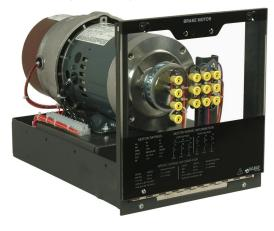
The Brake Motor (EMS Version) consists of a three-phase, fourpole, squirrel-cage induction motor equipped with a spring-set brake for holding and stopping (fail-safe). The motor is dual voltage and can operate at either a low-voltage or a high-voltage setting.
