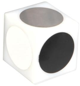
The Reflective Block consists of a block with various types of reflection surfaces: white, black, shiny metallic, matte black metallic, and retroreflective. The dimensions of the block are: 75 x 75 x 75 mm ( $3 \times 3 \times 3$  in).
