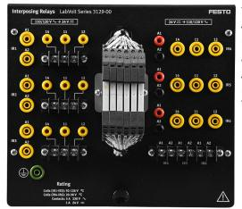
The Interposing Relays module consists of a bidirectional voltage converter for high and low control voltages. This model is equipped with three relays with 24 V dc coils and three relays with 110/120 V ac coils. Electrical connections for the low-voltage coils and contacts can be made using either the banana jacks or the terminal blocks.
