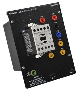
The Contactor consists of a three-pole contactor with a normally open auxiliary contact.
