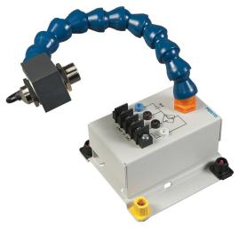
The Inductive Proximity Switch is sensitive to metals. The sensor is mounted on a flexible support for easy positioning. The model has one normally open and one normally closed contact, and the electrical connections are made using either the banana jacks or the terminal block.
