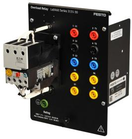
The Overload Relay consists of a three-phase, bimetallic overload relay with one normally closed and one normally open contact with an adjustable setting range.
