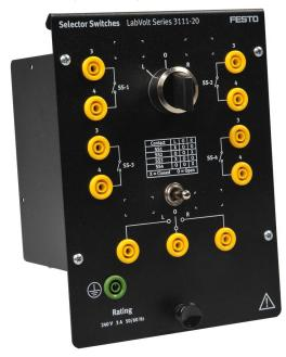
The Selector Switches module consists of a three-position, twopole selector switch and a single-pole double-throw toggle switch. It allows the user to alternate between two control circuit branches through the selector (at the top) or the toggle (at the bottom) switches. The two switches work independently. Selecting a position activates or deactivates the maintained contacts.
