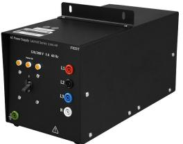
The AC Power Supply provides ac power for the Industrial Controls Training System. The outlet is fed from a three-phase, four-wire breaker panel supplied elsewhere. The power supply contains input and output pilot lamps, two "on-off" switches and dual sets of four color-coded banana jacks for three-phase voltage. All outputs are circuit-breaker protected. The AC Power Supply mounts on the upper shelf of the Mobile Workstation, Model 3103-4, and can provide power to both sides of the workstation.
