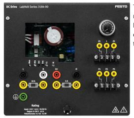
The DC Drive consists of a pulse-width modulated (PWM) dc motor speed control with maximum and minimum speed, current limitation, and IR compensation adjustments. Some electrical connections can be made using either the banana jacks or the terminal blocks.
