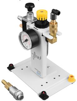
The Conditioning Unit (Single Port) conditions and regulates the pressure of the air supplied to the pneumatic circuits. It consists of a main shutoff valve, filter, a pressure regulator, pressure gauge, sleeve valve, and a muffler. The Conditioning Unit (Single Port) requires compressed air from a central air supply or a portable unit.
