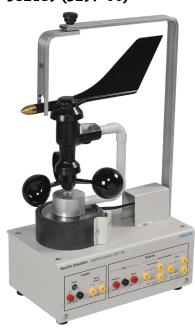
The Nacelle Simulator replicates the main functionalities of a wind turbine. It is designed to measure the speed and direction of the wind so that a PLC can control the position of the nacelle to optimize its operation. Two limit switches with NO and NC contacts allow monitoring of the number of rotations of the nacelle.
