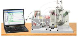
The Electro-Pneumatic Training System uses a PLC to control a variety of pneumatic industrial applications.
