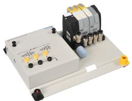
The Electro-Pneumatic Valve Island comprises two 4-way/2-position valves with common input and exhaust ports. One valve is operated by two solenoids and the other by a single solenoid and a spring return. The solenoids are actuated by 24 V dc signals.
