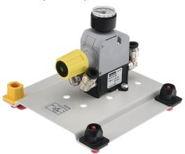
The Pressure Regulator offers two different air flow paths: one not regulated and one limited in pressure. A rotary knob and an air gauge make it simple to regulate the pressure to the desired value, thus limiting the pressure sent to the Electro-Pneumatic Training System, Model 8075-2.
