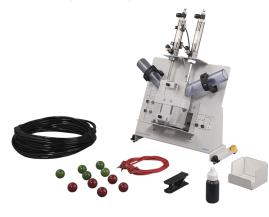
The Electro-Pneumatic Module and the associated equipment enable stamping, hold-and-punch, and filling operations. The module features two pneumatic cylinders arranged so as to distribute a programmed number of marbles from two tubes (feed lines) into a container. A second configuration allows students to perform a clamp-and-work operation on a plane material, such a sheet of paper. Two reed switches and one limit switch are installed to provide feedback on the cylinders' positions.
