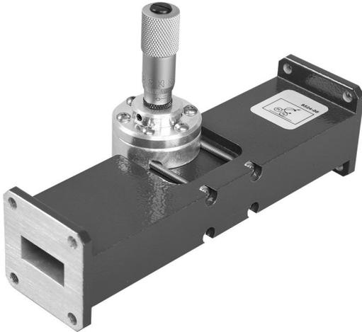
The Resonant-Cavity Frequency Meter is a device used in the Microwave Training System to perform frequency measurements.
