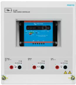
The DC 48V PWM Charge Controller is one of the most popular charge controller types. Although it is not the most efficient controller type, it is attractive to consumers due to its low price. The DC 48V PWM Charge Controller must be used in conjunction with the 48V Lead-Acid Battery Pack and solar panel emulator.
