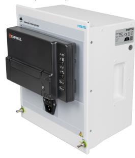
The communications gateway is an A4 module that is used to communicate and set grid-tied inverters over the AC line voltage directly. The gateway is connected on the AC line voltage just like the inverters it needs to communicate with. Using that line voltage, the gateway monitors the grid-tied inverters operation and enables the user to program them with specific operating parameters.
