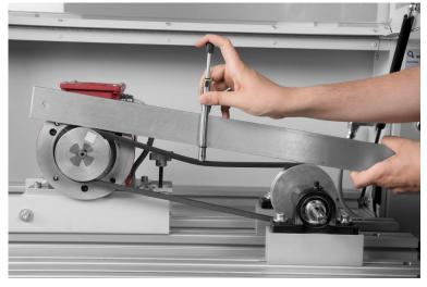
Properly aligned pulleys, sprockets, and gears as well as adjustment of belt tension, chain slack and gear backlash are essential in mechanical drives. The Level 1 package includes hardware and tools to master these skills.
