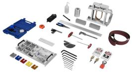
The Mechanical drives training system is a turnkey solution. Instructors will find most fasteners, tools, and measuring apparatus required for the suggested experiments in the Workstation Accessories package.
