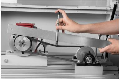
Properly aligned pulleys, sprockets, and gears as well as adjustment of belt tension, chain slack and gear backlash are essential in mechanical drives. The Level 1 package includes hardware and tools to master these skills.
